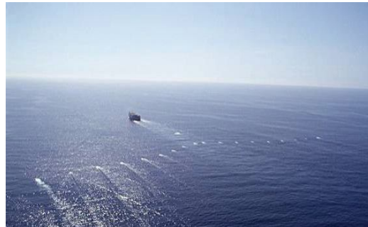
Fig. 1. One of the world’s most efficient seismic data gathering machines in action. In this case it tows 16 cables with a length of 4 kilometers. The whole spread is around 1.5 kilometers wide. The air bubble from the last shot can also be seen.
