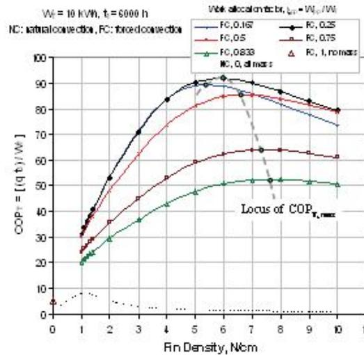
Fig. 1.  $COP_T$  for rectangular plate-fin arrays.  $W_T = 10 \text{ kWh}$ , regular duty cycle,  $t_1 = 6000 \text{ h}$  {3 years, 50 wk., 5 days/wk., 8 h/day},  $L = 0.1 \text{ m}$ ,  $W = 0.1 \text{ m}$ ,  $H = 0.05 \text{ m}$ ,  $\theta_B = 25 \text{ K}$ , aluminum.
