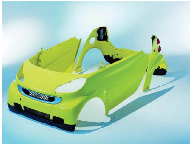
Figure 5. PP-based body panel system for the SMART for two lightweight passenger car (Daimler AG, Germany).
