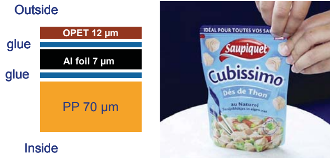
Figure 2. Typical construction for sterilizable SUP film laminate (OPET – oriented poly (ethylene terephthalate), Al – aluminium, PP – polypropylene) and application example highlighting user comfort.
