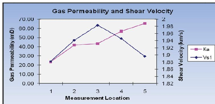
Figure 11. Gas Permeability and Shear Velocity Plot for Sample #12. From this chart, the relationship of permeability and shear velocity measured at the same location is not apparent. The trend is clear if you consider measurement locations #3, 4, and 5. Whereas, the trend is not present in measurement locations #1 and 2.
