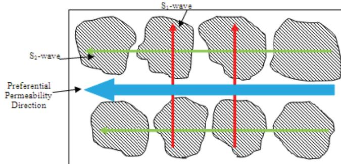
Figure 10. S1-wave propagating perpendicular to preferential permeability direction, and S2-wave propagating parallel to preferential permeability direction.
