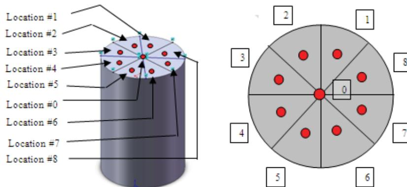
Figure 1. D view and Top view of permeability measurement points on a core sample.
