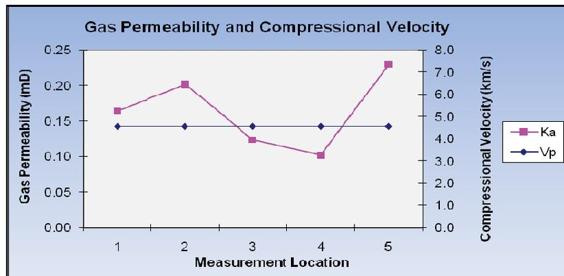
Figure 7. Gas Permeability and Compressional Velocity Plot for Sample #1. It is apparent from this chart that when permeability changes from one location to another on the sample, compressional wave velocity does not reflect that change.
