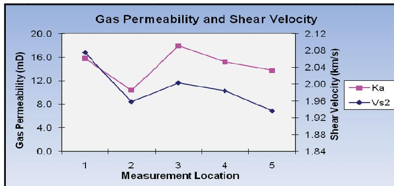
Figure 9B. Gas Permeability and Shear Wave Velocity Plot for Sample #5. It is apparent from this chart that a proportional relationship may exist between permeability and shear wave velocity ( $S_2$ -wave) measured at the same location.
