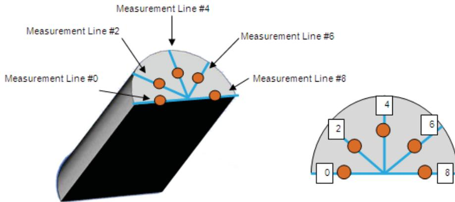
Figure 4. 3D view and Top view of velocity measurement lines on a core sample
