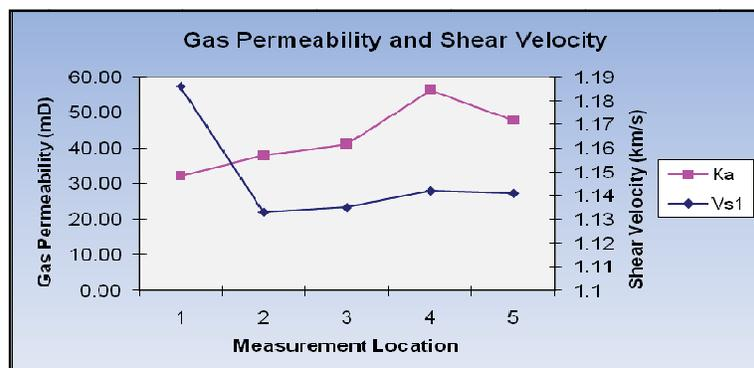
Figure 12. Gas Permeability and Shear Velocity Plot for Sample #15. From this chart, the relationship between permeability and shear velocity measured at the same location does not exist. This is probably due to the random or more complex distribution of permeability within the sample.
