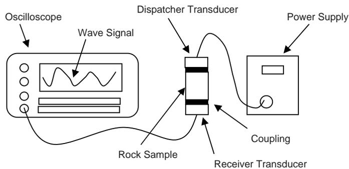
Figure 5. The setup used to conduct velocity measurements on each measurement line shown in Figure 4.
