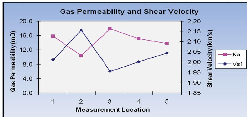
Figure 9A. Gas Permeability and Shear Wave Velocity Plot for Sample #5. It is apparent from this chart that an inverse relationship may exist between permeability and shear wave velocity ( $S_1$ -wave) measured at the same location.
