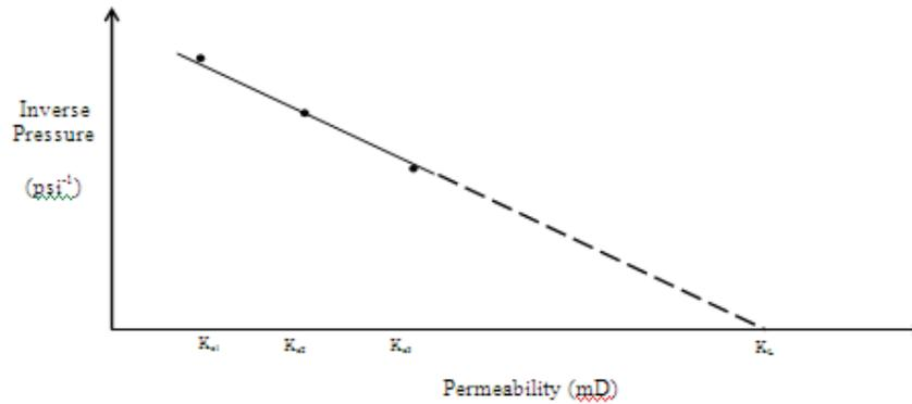
Figure 2: Estimating liquid permeability from gas permeability (Klinkenberg Effect)
