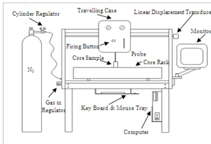
Figure 3. The main components of PDPK are Table and Frame, Travelling Case, Core Rack, and External Nitrogen Computer.
