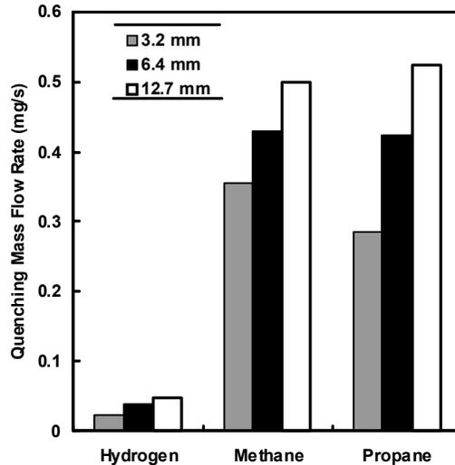
Figure 11. Quenching limits for leaky compression fittings for tube diameters of 3.1 mm, 6.3 mm and 12.6 mm. The fittings were vertically oriented and upstream absolute pressure was 4 bar.
