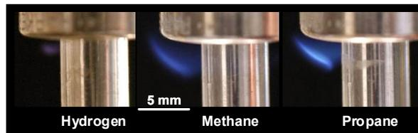
Figure 8. Flames near extinction on leaky compression fittings for hydrogen, methane, and propane (original in color). Also visible here is the 6.3 mm tube and the threaded nut. The fitting was vertically oriented and the upstream absolute pressure was 4 bar.
