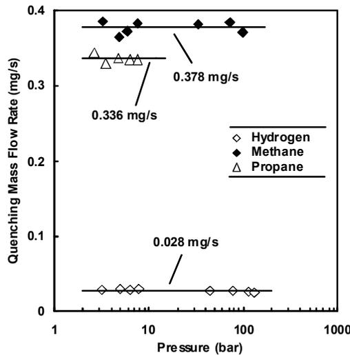
Figure 9. Quenching limit (minimum flaming flow rate) versus upstream absolute pressure for a 6.3 mm leaky compression fitting in the vertical orientation. The line fits represent mean values of the measured quenching limits.
