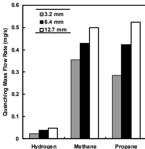
Figure 11. Quenching limits for leaky compression fittings for tube diameters of 3.1 mm, 6.3 mm and 12.6 mm. The fittings were vertically oriented and upstream absolute pressure was 4 bar.
