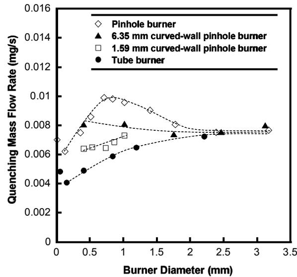
Figure 4. Quenching mass flow rates for hydrogen for various burner types and diameters.
