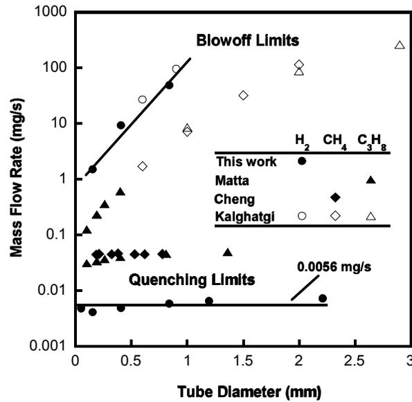
Figure 3. Quenching and blowoff limits for tube burners. Hydrogen quenching and blowoff limits include best fit lines. Past measurements shown are from [13,14,19].
