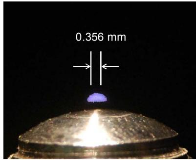
Figure 2. Color image of a hydrogen flame slightly above its quenching limit of  $7.5 \mu\text{g/s}$ . The burner is a 0.36 mm pinhole burner and is oriented vertically. The image was recorded in a dimly lit room at  $f/4.2$  with an exposure time of 30 s.
