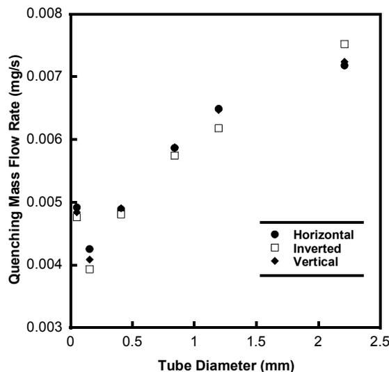
Figure 5. Quenching mass flow rates for tube burners in horizontal, inverted, and vertical orientations.
