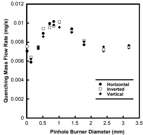
Figure 6. Quenching mass flow rates for pinhole burners in horizontal, inverted, and vertical orientations.
