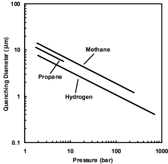
Figure 7. Minimum diameter of a circular port for flaming (quenching diameter) as a function of upstream absolute pressure assuming isentropic choked flow.
