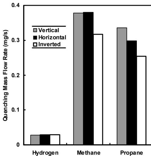
Figure 10. Quenching limits for a 6.3 mm leaky compression fitting in vertical, horizontal and inverted orientations. The upstream absolute pressure was 4 bar.
