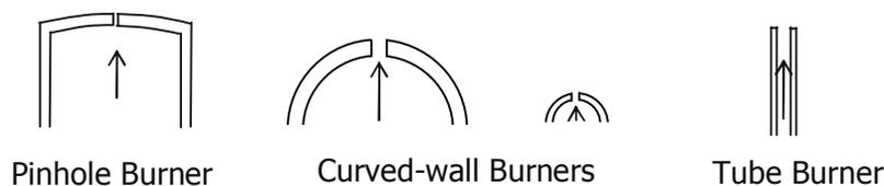
Figure 1. Schematics of the present round-hole burners. Arrows show the fuel flow direction. Burner dimensions are given in Table 2.
