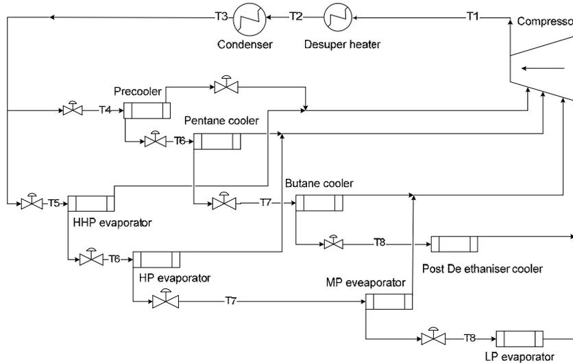
Figure 6. Propane cycle block diagram.
