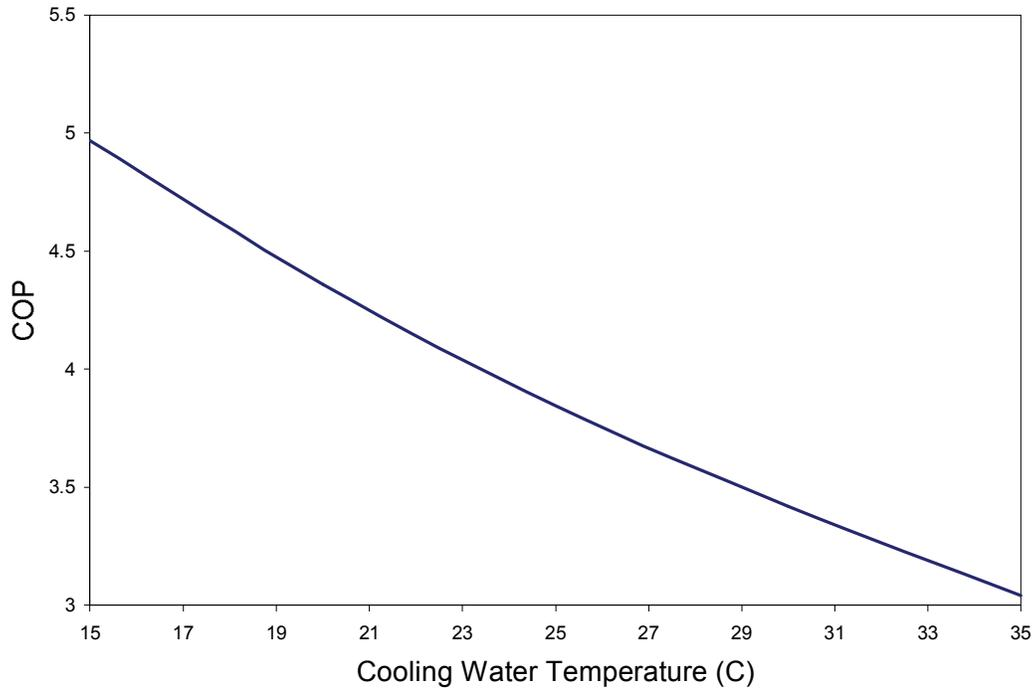
Figure 8. Predicted effect of cooling water temperature on total COP.
