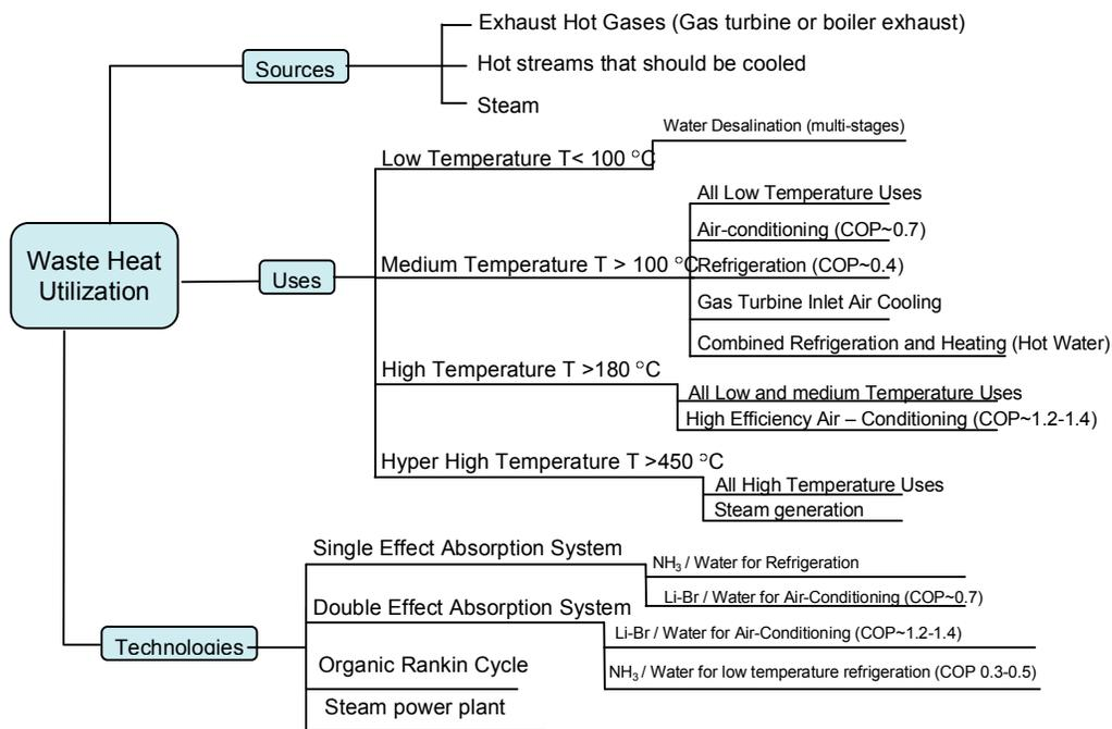
Figure 1. Waste heat utilization evaluation steps in terms of sources, uses, and technologies.
