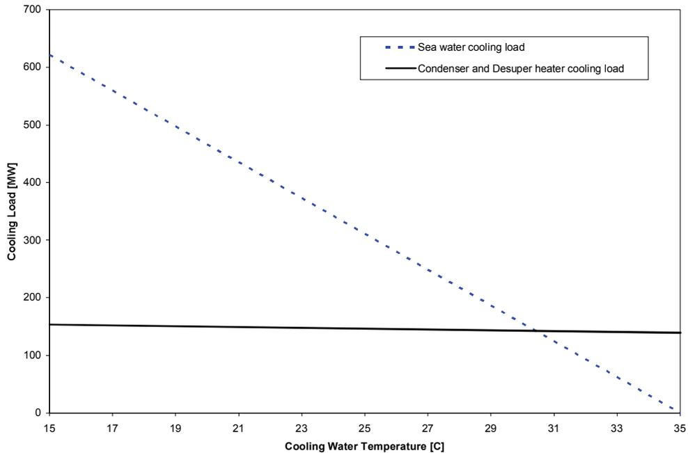
Figure 7. Predicted amount of cooling needed for cooling sea water from 35 °C to condenser cooling water temperature and condenser and desuper heater cooling load.
