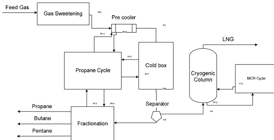
Figure 2. Schematic illustration of an LNG plant-process.
