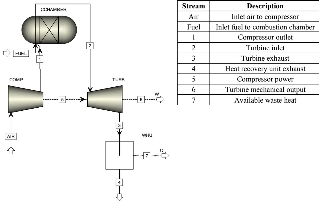
Figure 3. ASPEN block diagram of the gas turbine model.
