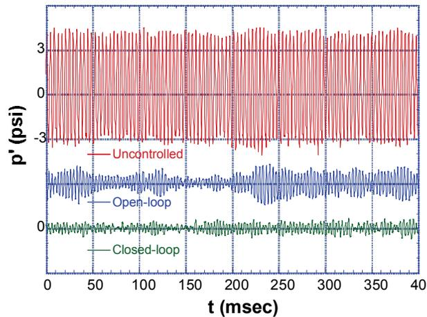
Figure 1. Comparison of uncontrolled and controlled pressure oscillation amplitudes [2].
