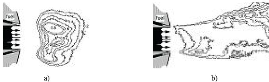
Figure 2. Actively controlled diffusion flames, a) efficient and b) sooty flames [3].
