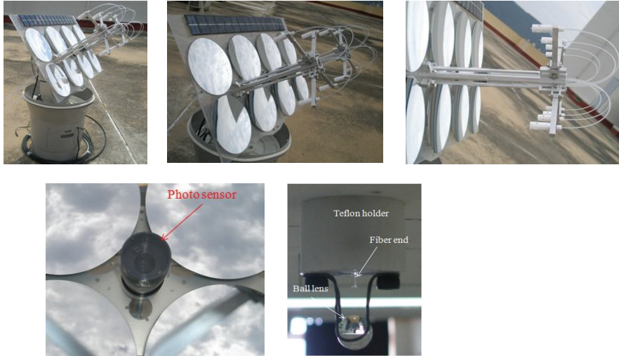
Figure 3. Photographs of homemade fiber optic solar lighting system.
