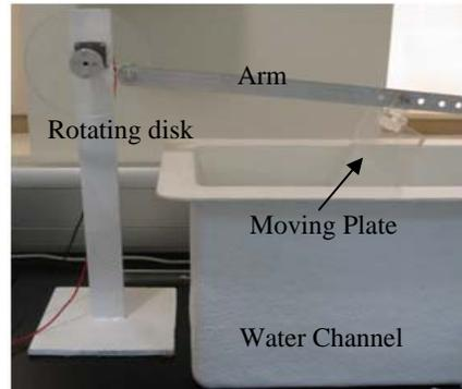
(b) The wave generator is to produce ripples in the water surface resulting in waves
