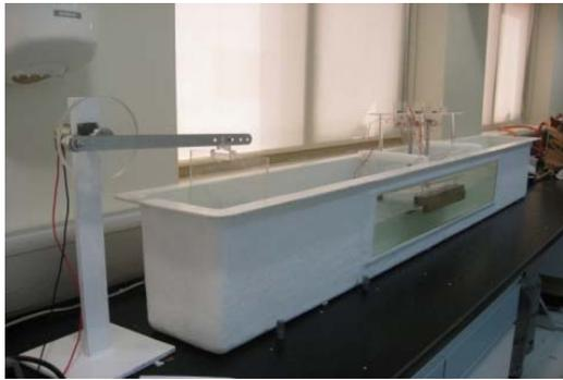
(a) The laboratory scale water channel with transparent windows for flow visualization
