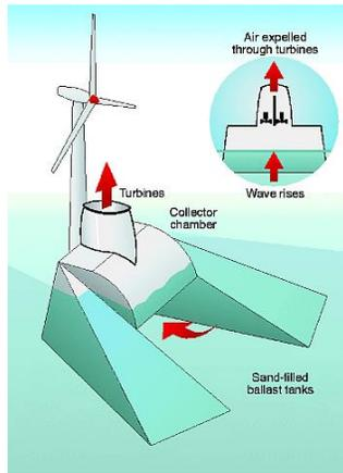
a) Wave-powered electricity generator [3]
