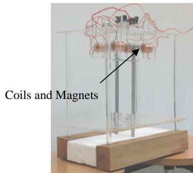
(c) The power generator which operates based on Faraday induction consists of 4 sub-parts
