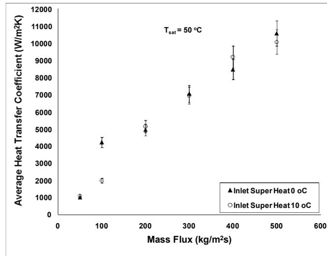
Figure 21. Effect of mass flux on average heat transfer coefficient R245fa at  $T_{sat} = 50^{\circ}\text{C}$ .
