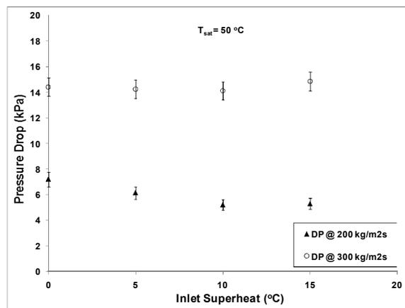
Figure 19. Effect of inlet superheat on pressure drop at  $T_{sat} = 50^\circ\text{C}$  for R245fa.
