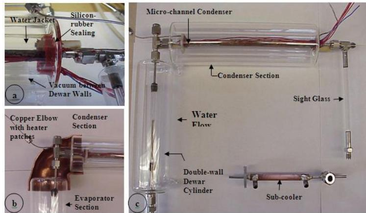
Figure 13. Details of test section, (a) details of the joint between the condenser section and sight-glass, (b) details of the joint between the evaporator Dewar and condenser Dewar, and (c) view of the arrangement of various parts in the refrigeration loop.
