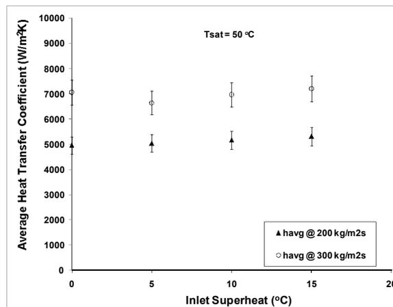
Figure 17. Effect inlet superheat on average heat transfer coefficient at  $T_{sat} = 50^\circ\text{C}$  for R245fa.
