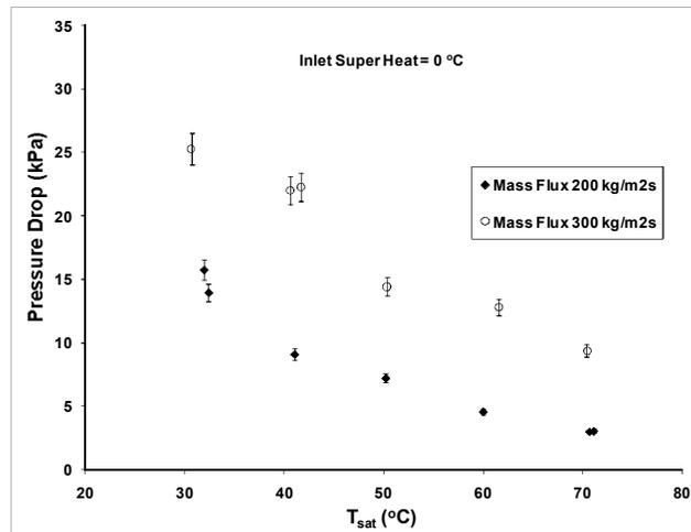
Figure 27. Effect of saturation temperature on pressure drop for R245fa.
