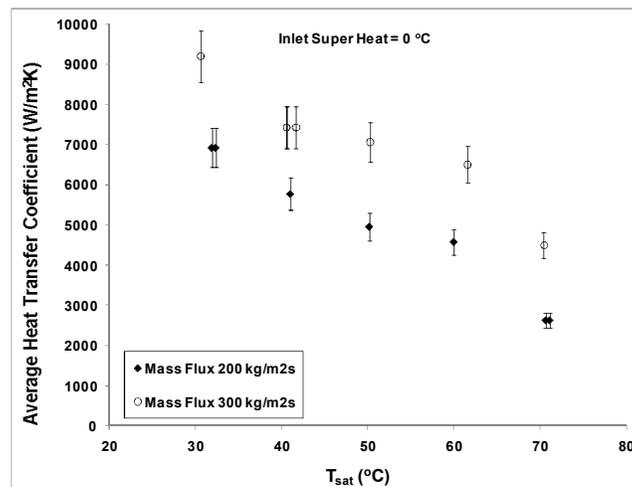
Figure 25. Effect of saturation temperature on average heat transfer coefficient for R245fa.
