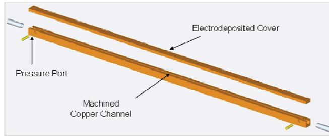
Figure 14. A drawing of the fabricated micro-channel.
