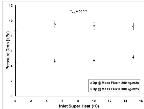
Figure 18. Effect of inlet superheat on pressure drop at  $T_{sat} = 50^\circ\text{C}$  for R134a.
