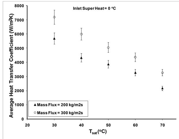
Figure 24. Effect of saturation temperature on average heat transfer coefficient for R134a.
