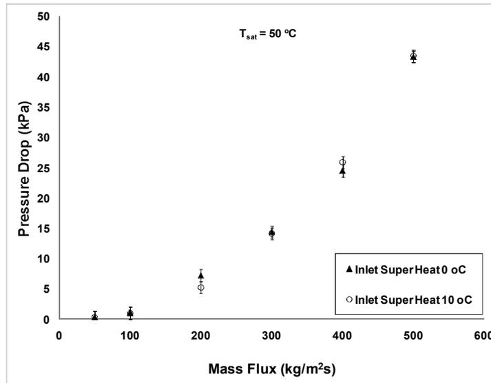
Figure 23. Effect of mass flux on pressure drop R245fa at  $T_{sat} = 50^{\circ}\text{C}$ .
