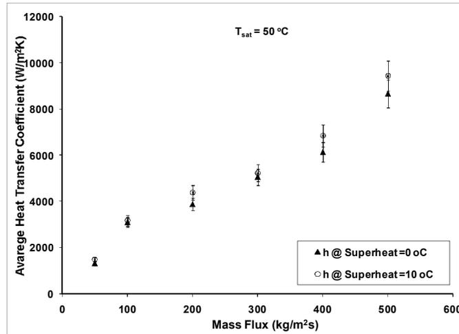
Figure 20. Effect of mass flux on average heat transfer coefficient for R134a at  $T_{sat} = 50^{\circ}\text{C}$ .
