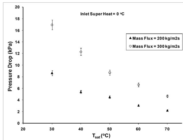
Figure 26. Effect of saturation temperature on pressure drop for R134a.
