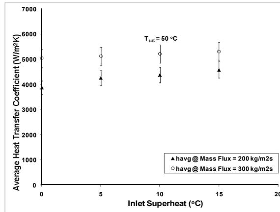
Figure 16. Effect of inlet superheat on average heat transfer coefficient at  $T_{sat} = 50^\circ\text{C}$  for R134a.
