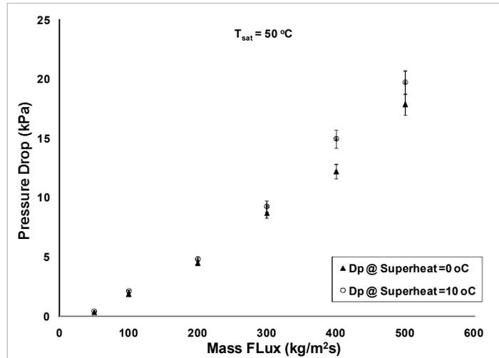
Figure 22. Effect of mass flux on pressure drop R134a at  $T_{sat} = 50^{\circ}\text{C}$ .
